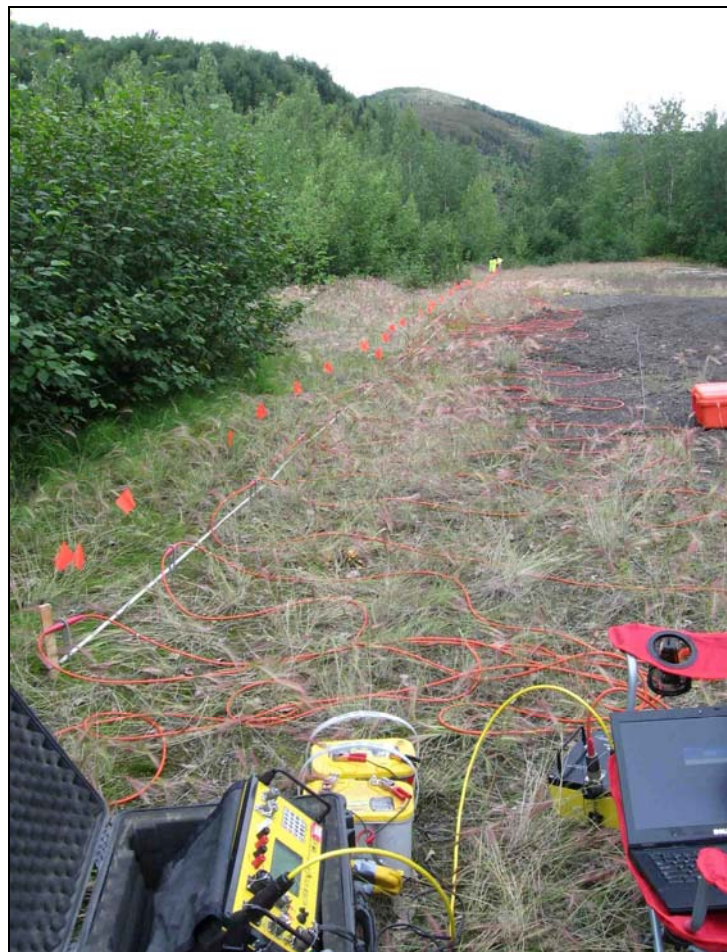
Figure 12. Photograph of the DC resistivity equipment deployed on line 4 across the pre-1955 retort area, looking southwest.
