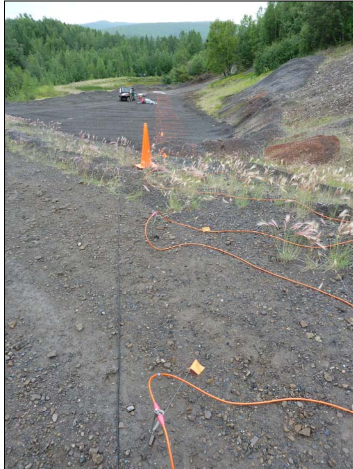
Figure 5. Photograph of the DC resistivity equipment deployed on line 1, looking northeast toward settling pond #1.
