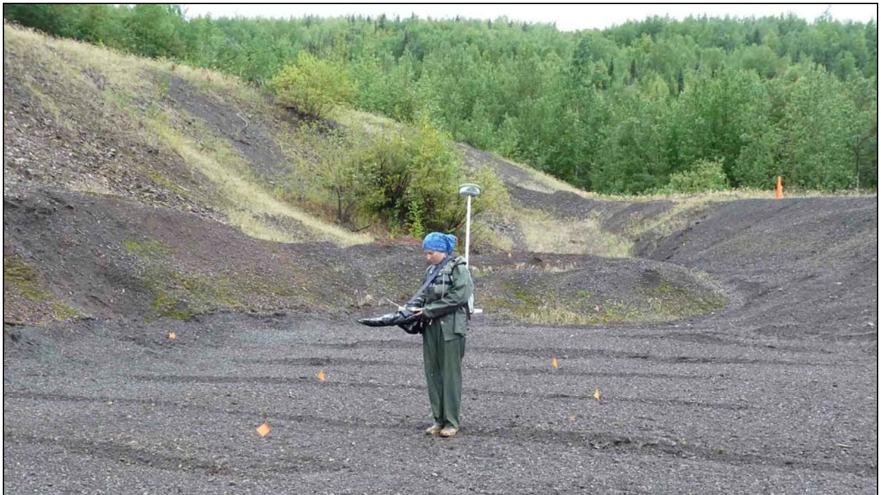
Figure 4. Photograph of the shoulder-slung electromagnetic induction system in horizontal co-planar mode integrated with a backpack-mounted global positioning system. The operator is standing at the calibration station facing north.
