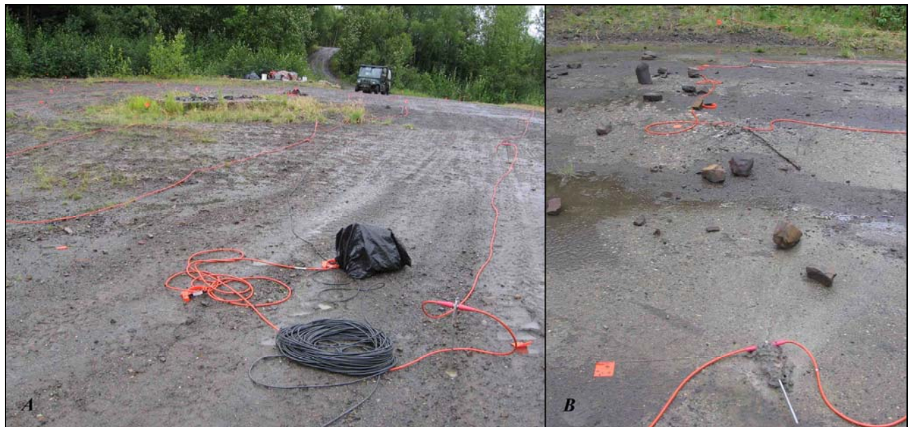
Figure 14. Photographs of the (A) DC resistivity equipment deployed on the three-dimensional grid across the pre-1955 retort area, from the southeast corner of the grid looking northeast and (B) the three electrodes along the southwest edge of the grid placed on the concrete using bentonite mud, looking northwest.
