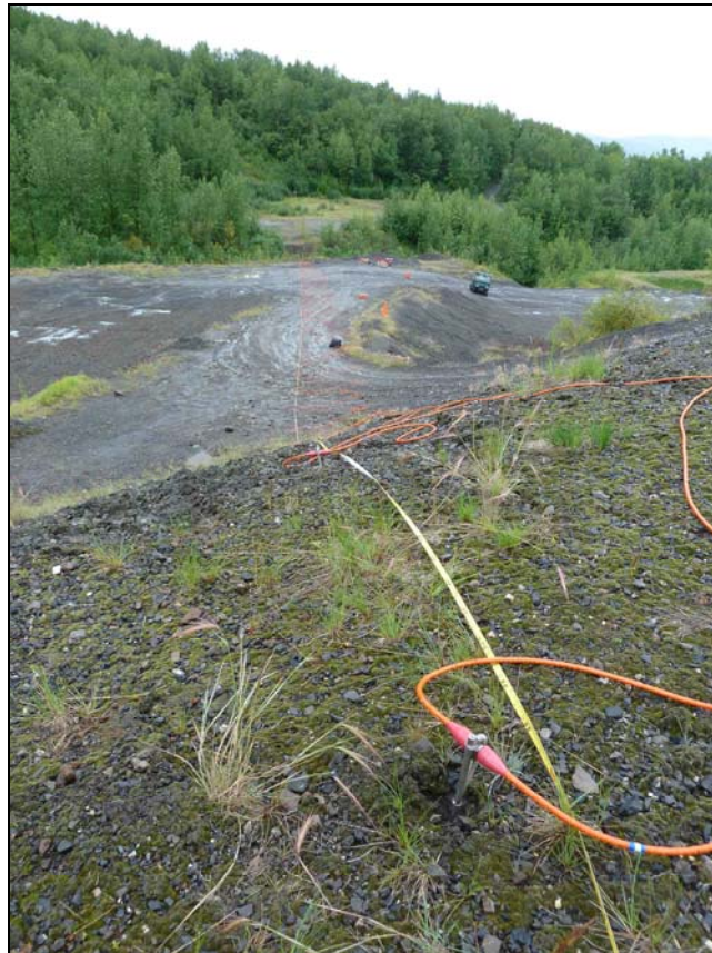
Figure 7. Photograph of the DC resistivity equipment deployed on line 2a taken from monofill #2, looking northwest.
